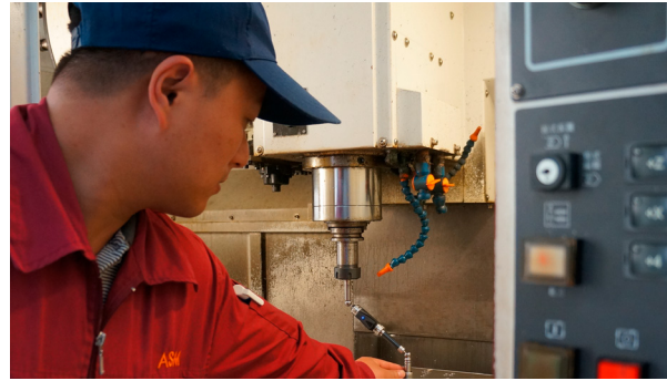
ASMT's production staff regularly calibrate their CNC machine tools
